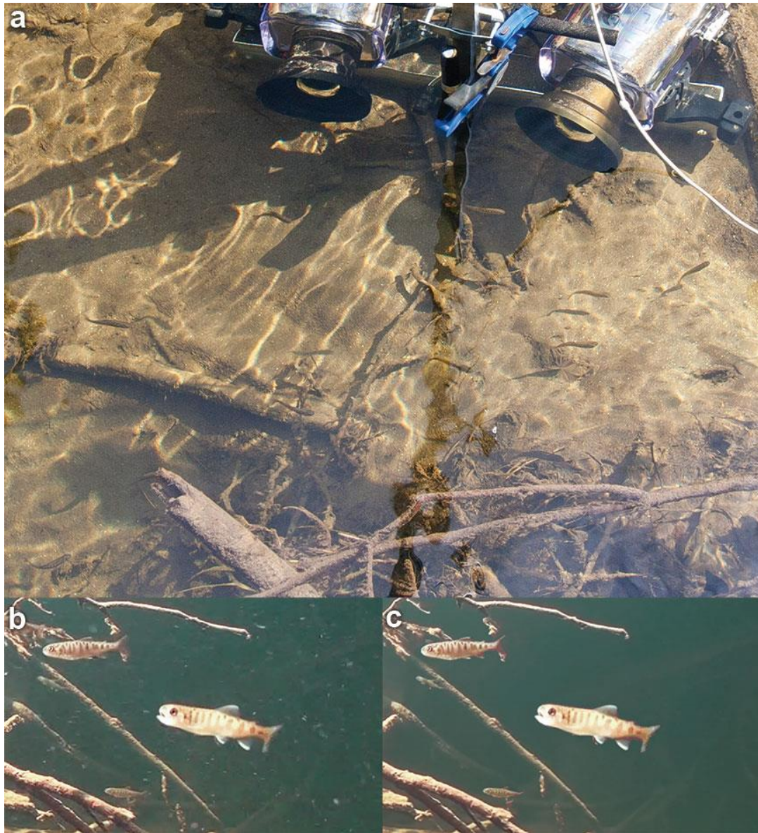
Fig. 2.1. Videotaping fish amidst debris in clear water. (a) The 0.7-m deep water appears crystal clear from above; however, (b) it carries numerous fine debris particles, evident in comparison to (c) a version of the same image with the debris removed by averaging several video frames.
