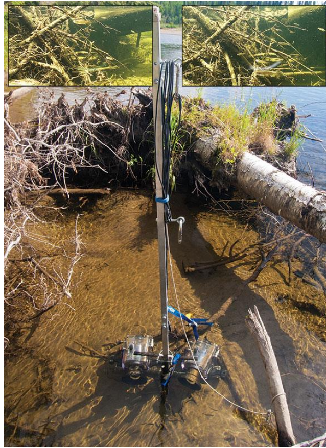
Fig. 1.6. Deployed stereo camera system. Also shown is each camera's view of a rootwad and associated juvenile Chinook salmon. In this slow-water set, the blue ratchet strap attached to a log behind the cameras was sufficient to hold them steady. Some extraneous attachments are visible, but are not described in our text because they are not all necessary and will vary with each study's needs.
